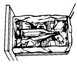
Bottles or cans not placed in the center may become caught between the ram and the drawer. The Drawer Monitor Switch senses a "misload" and causes the ram to return to the "up" position without compacting. Load bulky trash, bottles and cans in the **center** of the drawer.
